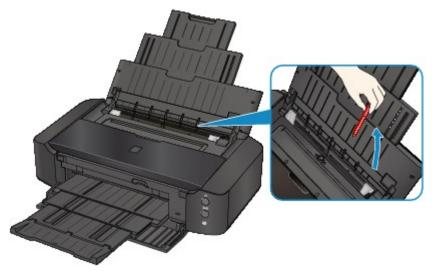
Check7 Make sure that the disc tray guide is closed completely.
