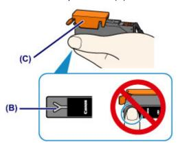
3. Lift up the tab on the orange protective cap (C) to remove it off GENTLY.
