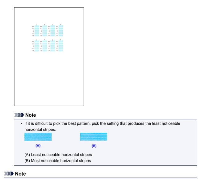
• After head alignment is completed, you can print and check the current setting. To do so, click the **Print Head Alignment** icon and when the message is displayed, click **Print Alignment Value**.
