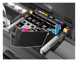
2. Press on the top of the ink tank until the ink tank snaps firmly into place.
